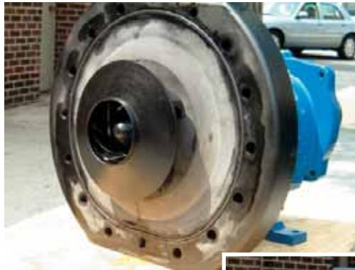
A 4 x 3 - 9 chemical pump with an enclosed impeller instead of an open impeller.
