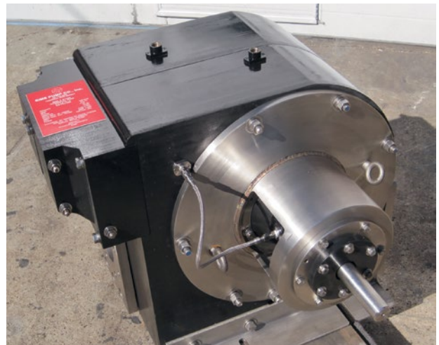
Image 4. This composite pump was re-engineered into a two-stage structural composite pump with single-suction impellers. It is approximately 11 percent more efficient than the original metallic pump (before corroding).
