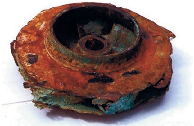
Image 3. Damage from corrosion, erosion and cavitation can quickly destroy metallic pumps and pump parts.
