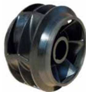
This structural composite double-suction impeller machined from a solid block of composite replaces a cast bronze impeller for a main sea water cooling pump.
